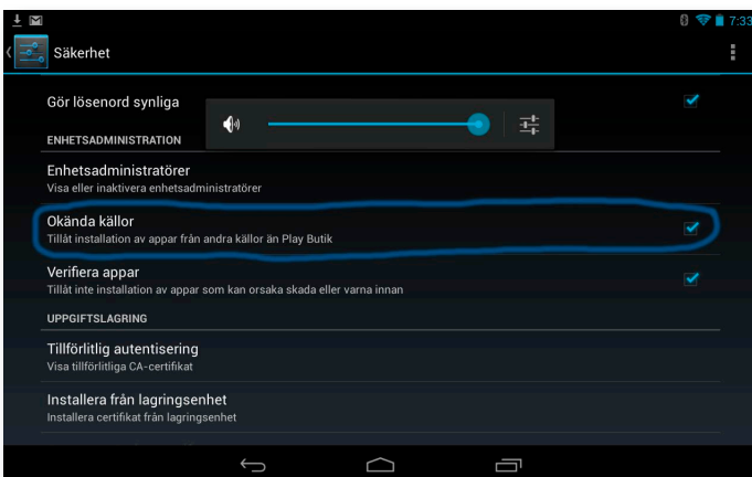
Fig 3e - MDash is not currently available on Google Play but only available for download directly from www.maxxecu.eu After downloading the app, simply approve "install from unknown sources". Activation of this is done in Android's settings, Security and "Unknown sources" ["Allow installation of applications from unknown sources"].
